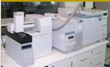
Headspace gas chromatograph mass spectrometer
